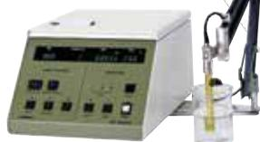
Model F-80 (benchtop) The world's first instrument capable of measuring pH at 1/1000 resolution, includes an integral computer, with automatic calibration and a self-diagnostic function.
