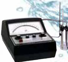
M-5 (benchtop) From a vacuum tube to a semiconductor, allowing miniaturization and fast response.
