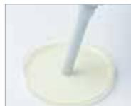
The sensor is located on the flat surface of the electrode tip, with less than a 100 µm protrusion from the housing.
