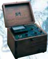
HORIBA introduces Japan's first glass electrode pH meter.
