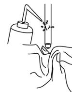
**2. Open the internal solution filler port of the pH electrode.**
