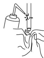
2. Open the internal solution filler port of the pH electrode.
