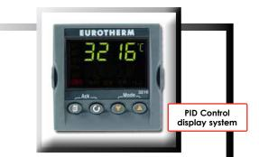
Controller – A digital microprocessor based PID temperature controller controls the temperature within the range ambient +5°C to 200°C, temperature fluctuation at 105°C is ±1°C.
