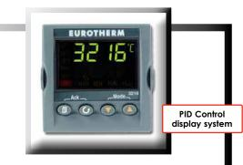
Controller – A digital microprocessor based PID temperature controller controls the temperature within the range ambient +5°C to 300°C, temperature fluctuation at 105°C is ±1°C.
