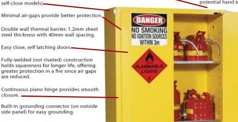
Dual vents with builtin flame arresters strategically placed at bottom and opposite top are welded, not screwed in place.
