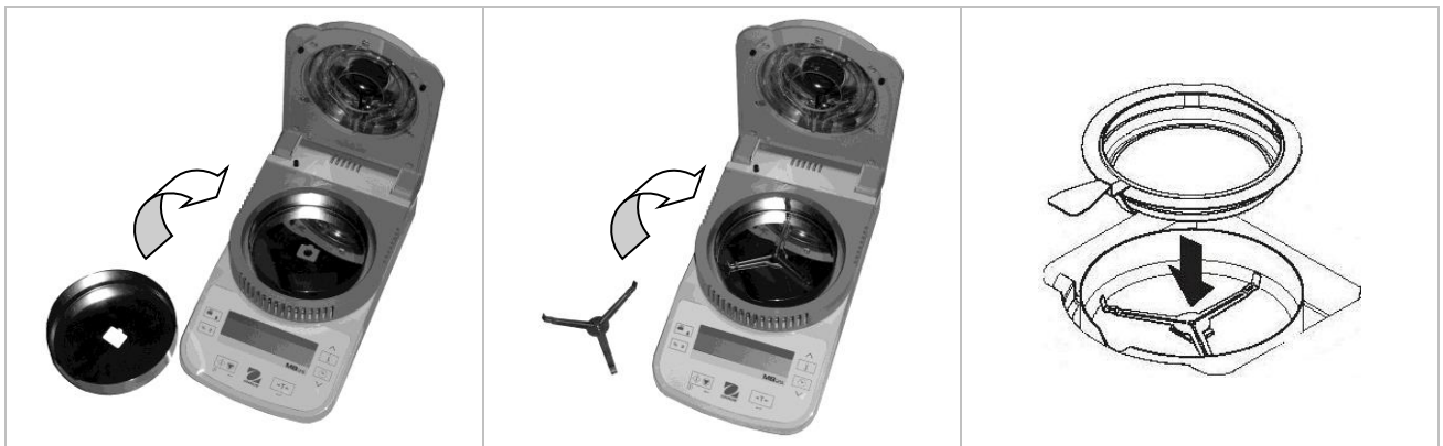
(1) Install and position Draft Shield
