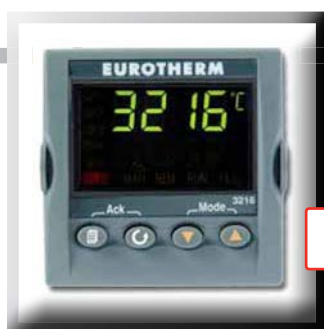
PID Control display system
