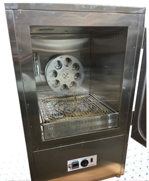
Inside the working chamber of RTFO24 with bottom mounted controls
