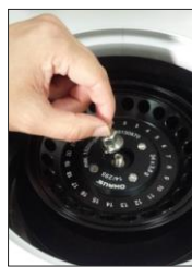
Rotor with separate nut
