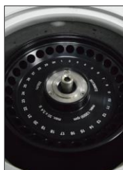
Rotor with built-in nut
