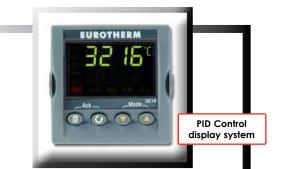
Controller – A digital display temperature controller controls the temperature within the range ambient +5°C to 300°C.
