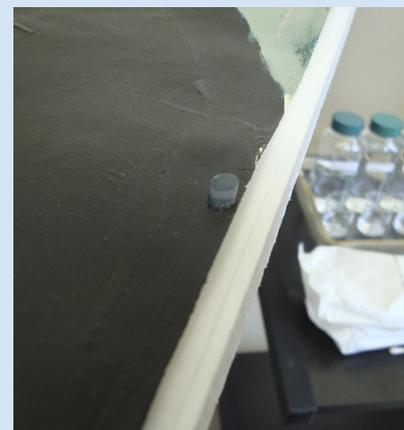
Figure 1: An agarose pellet resting on the surface of an acrylic paint film.
