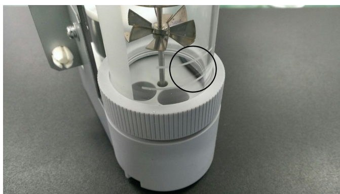
Fig. 125 Packing runs off the inside of the extraction tank
