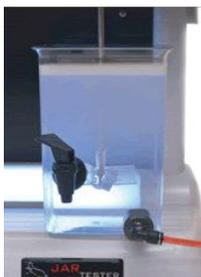
2L DAF Jar contents under flotation with an axial flow propeller type paddle in place
