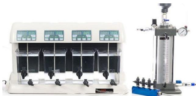
2L capacity DAF Saturator, distribution Manifold, 4 x 2L DAF Jars and hoseware
