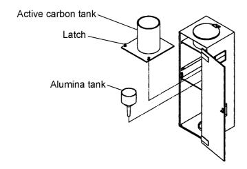
3. Fill the alumina tank with all of alumina (90 g).
