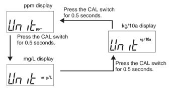
4. Press the MEAS switch to apply the setting.
