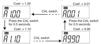
Press the MEAS switch to apply the setting. The measurement mode is returned.
