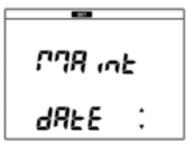
Press the ENTER key to enter the year setting screen. Press the ◄ or ► key to select a digit and press the ▲ or ▼ key to change the value, and then press the ENTER key.
