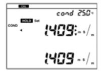
**8.** After the calibration is completed, press the MEAS key to return to the measurement screen.
