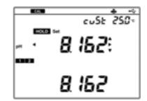
The **2** mark, which means that the second point calibration is completed, is displayed on the screen.
