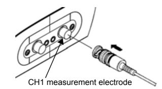
**2.** Turn the electrode connector to the right along the groove to plug the connector.
