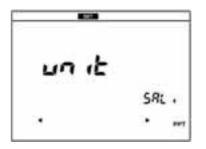
Press the ◀ or ► key to select PPT or %, and press the ENTER key.
