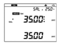
**8.** After the calibration is completed, press the MEAS key to return to the measurement screen.
