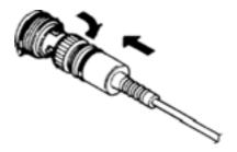
**3.** Put the connector cover on the connector.
