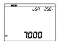
**6.** Check the stable indication value, and press the CAL key.
