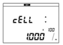
**2.** Press the ENTER key to enter the conductivity cell constant change screen.
