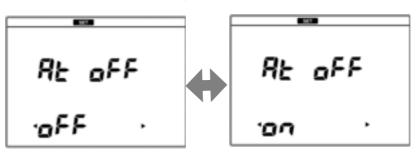
6. Press the ◀ or ▶ key to select a digit and press the ▲ or ▼ key to change the value, and then press the ENTER key and press the ENTER key to return to the auto power off change screen.
