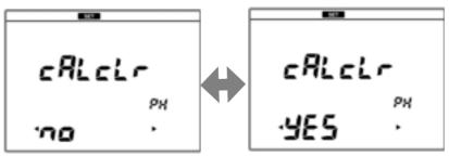
6. Press the ◀ or ▶ key to select Yes, and press ENTER key to delete the calibration data.
