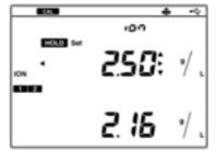
The **2** mark, which means that the second point calibration is completed, is displayed on the screen.
