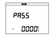
If this setting is ON, password entry is required when you power ON the instrument. Enter the password and press the ENTER key.
