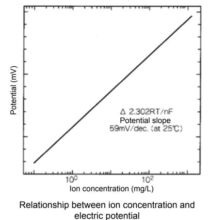
Calibration curve for univalent positive ion electrode
