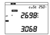
The **mark**, which means that the first point calibration is completed, is displayed on the screen.
