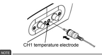
If the temperature connector is unconnected or the connection is wrong, the MTC set temperature is displayed as the sample temperature.
