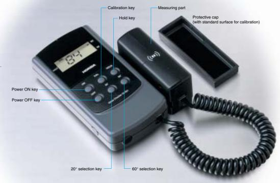
Guaranteeing uniform production quality and standards for gloss mesurement. HORIBA's IG Series Gloss Checkers display gloss measurements as numerical data, eliminating ambiguity and ensuring objective evaluation of a product's quality. Compact in design and ready when powered on, all the user needs to do is hold the portable gloss checker against the surface being evaluated for quality control of paints, polishes, floor maintenance and many other industrial applications.
