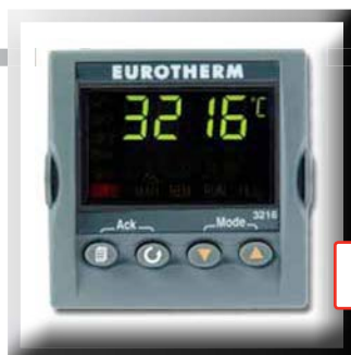
PID Control display system
