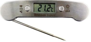
Foldable thermometer with stainless steel body (SS 304) and sensor probe, adjustable from 0 to 180 degrees, to allow different angle viewing. The probe folds away conveniently for easy storage when not in use. Suitable for a variety of uses including HVAC, food processing, agriculture, laboratory and energy management. Probe thermometers can be supplied with UKAS calibration certificate or statement of conformity on request.
